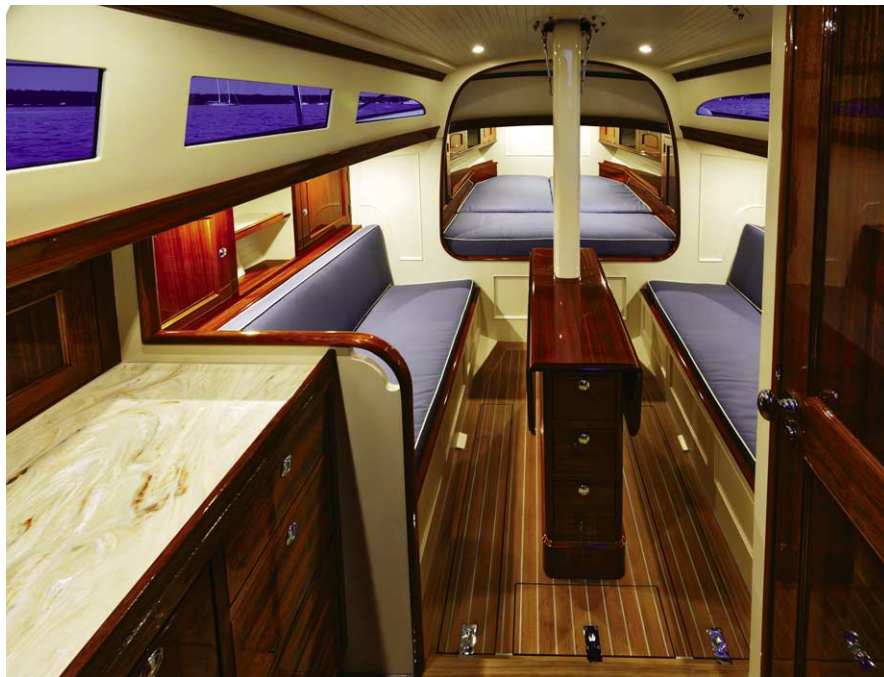
Wisp's interior furniture is built from sipo mahogany and includes a full queen berth forward.
