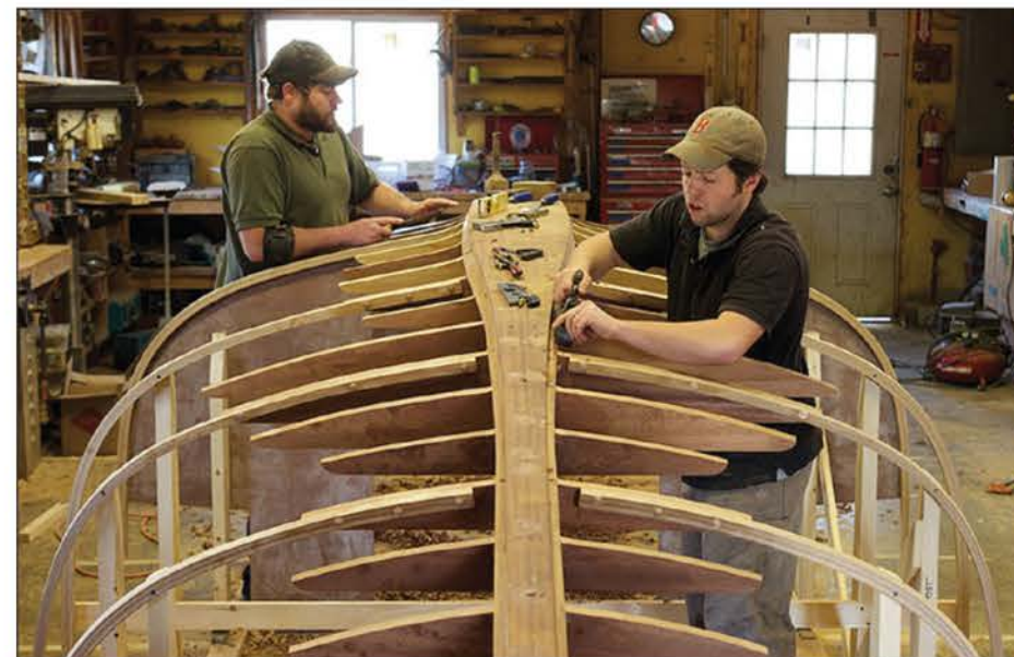
Artisan Boatworks craftsmen Ben Loveless (left) and Chad Meyers touch up the keel rabbet on UNCAS before they begin planking. For a detailed description of how these boats are built, see the article beginning on page 59.
