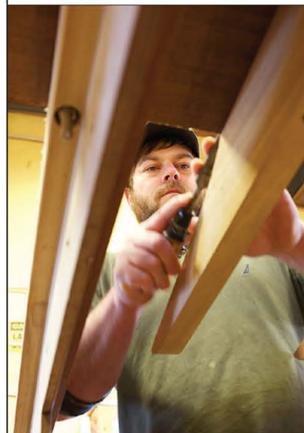
Ben Loveless touches up a floor timber prior to planking. "Alec's shop is perfect for shooting because of its size," says Alison. "There are varied heights giving me options for different angles and the walls are painted yellow, which gives a warm cast of lighting—which counterbalances the fluorescent lights nicely."
