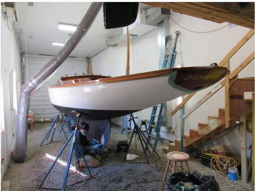
A worker applies paint to the hull of a sailboat within a paint bay at Artisan Boatworks on Jan. 16. (Photo by: Louis Bettcher)
