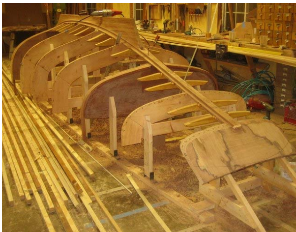
Fig. 23) MURMUR laminated mahogany keel & floors
