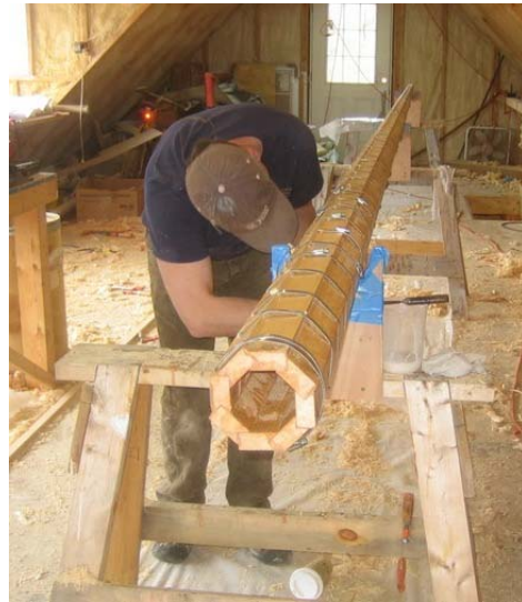
Fig. 50) Hollow “bird’s mouth” mast courtesy Artisan Boatworks
