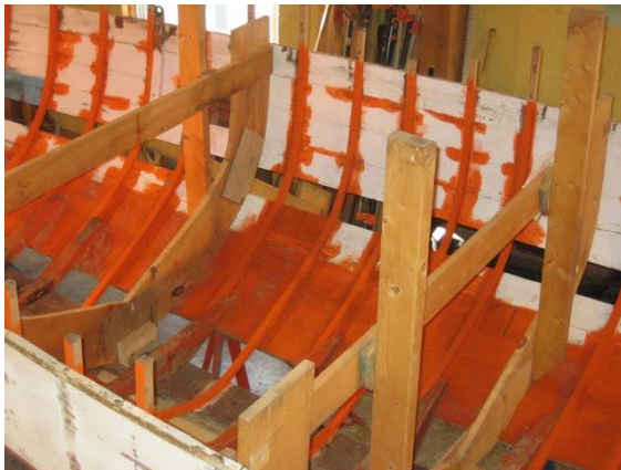
Fig. 15) New frames primed with red lead
