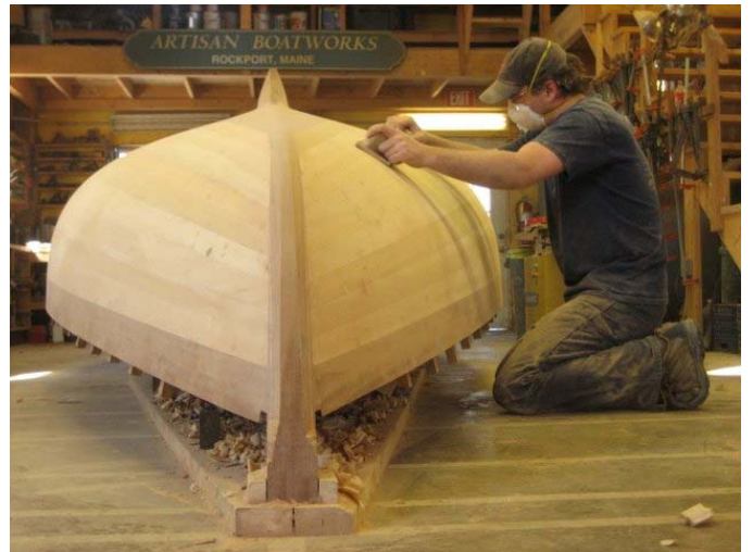
Fig. 28) MURMUR fairing with long-boards
