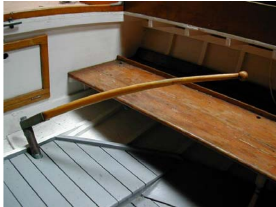
Fig. 56) Fixed tiller hardware - FLICKER courtesy Maynard Bray
