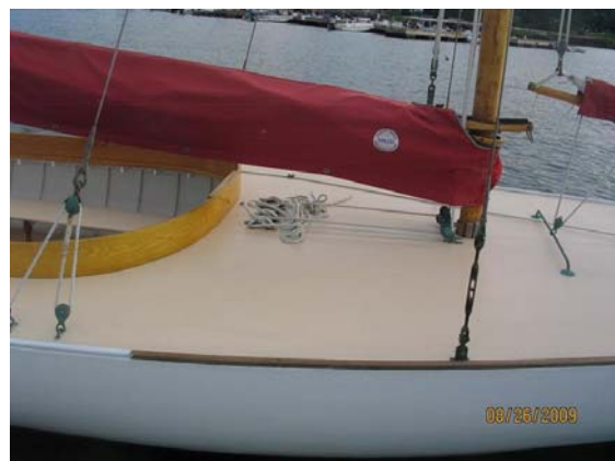
Fig. 42) Halyards moved forward courtesy William Beardsley
