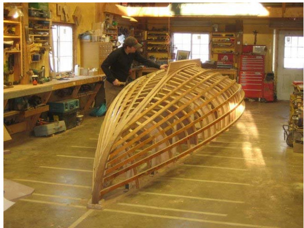
Fig. 24) MURMUR oak frames & "glu-lam" ribbands
