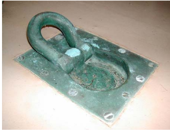
Fig. 62) FLICKER hoisting eye courtesy Maynard Bray
