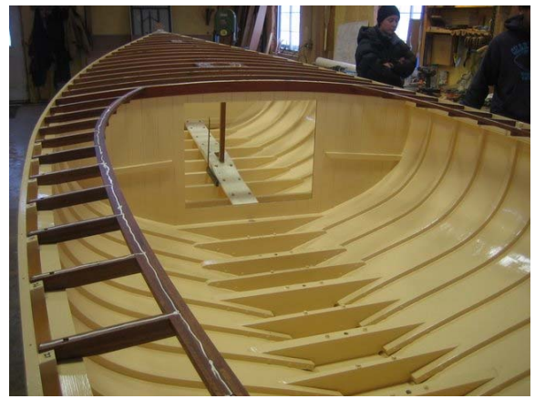
Fig. 30) MURMUR deck frame looking fwd
