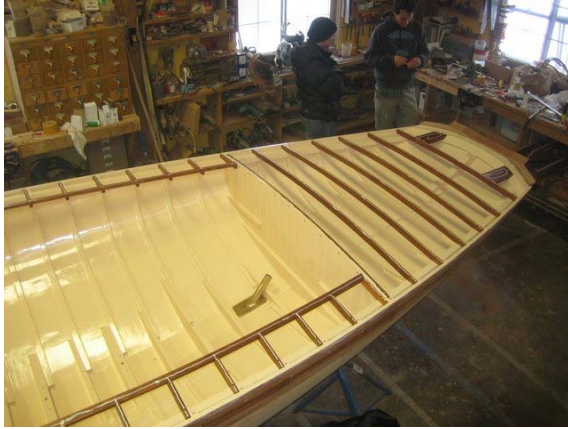
Fig. 31) MURMUR deck frame looking aft
