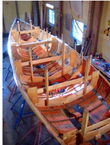
Fig. 14) Using molds to restore hull shape
