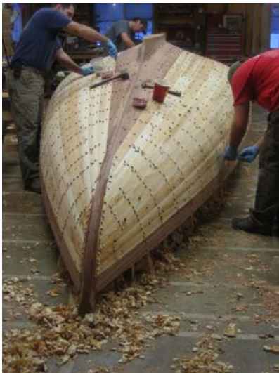
Fig. 27) MURMUR mahogany sheer planks/garboards
