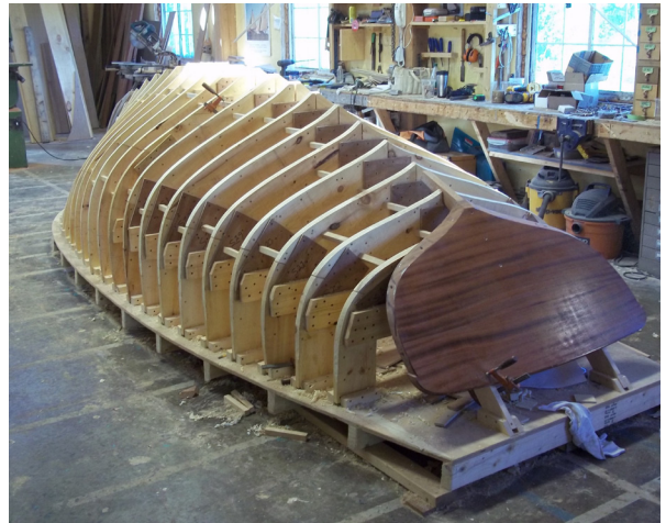
Building Jig for Herreshoff 12 1/2 replicas, with new transom in place.
