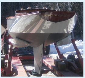
faired and epoxy coated, and the toe rails replaced. This proved to be a great example of how a wooden boat can be given an entirely new life, in a relatively straight-forward manner, for half the cost of a fiberglass replacement.
