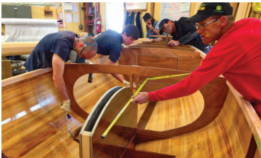
While the crew measures for deck beams and the centerboard trunk cap, the inside of the hull receives three coats of West System Epoxy, and then six coats of Epifanes varnish.
