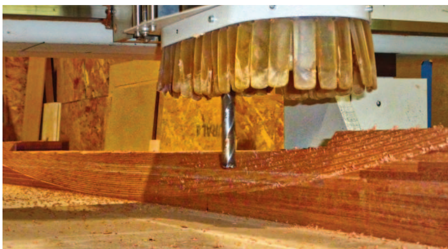
Many elements of the W-22 were produced using computer-assisted cutting, to save time and ensure consistency. In this photo, one half of the deadwood with centerboard slot is being machined from a 4-inch thick laminated mahogany blank.
