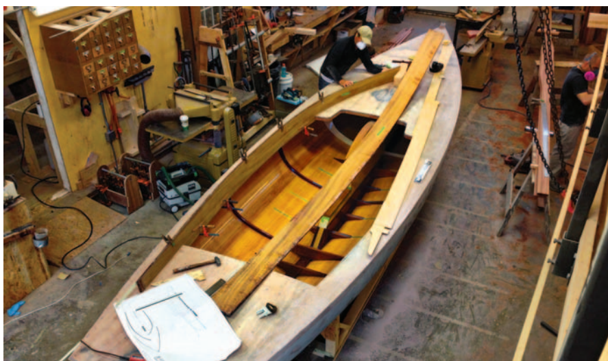
Chad Myers installs laminated teak coamings. The plywood deck is sheathed in 10 oz. fiberglass/epoxy.
