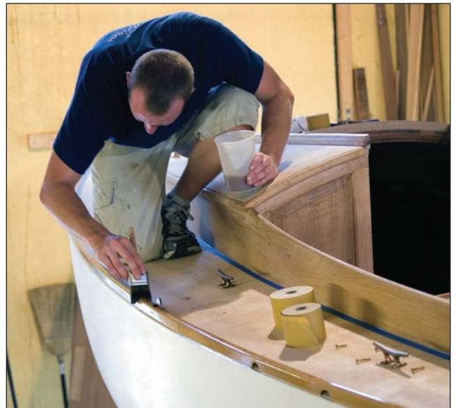
Top left—PHOENIX's plywood deck is sheathed in canvas set in a latex lagging adhesive. The coamings and cabinsides are continuous, and are built of steam-bent white oak. Chad Myers is installing hardware. Top right—Josh Howard paints the cockpit, whose sole will later be planked in \frac{1}{4} " teak. Bottom left—As PHOENIX awaits launching, Alec's wife, Erin, speaks with Jane and Bill Saltonstall. Above—Dave Ericson tends the brightwork.
