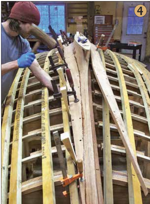
Photograph 4 —Wedges are driven between a hefty ribband and the glued-in-place garboard, driving the plank tight into the keel rabbet. Photograph 5 —The cedar broadstrake is glued and screwed in place. Photograph 6 —Excess glue is cleaned from the interior as well as from the limber holes in the floor timbers.
