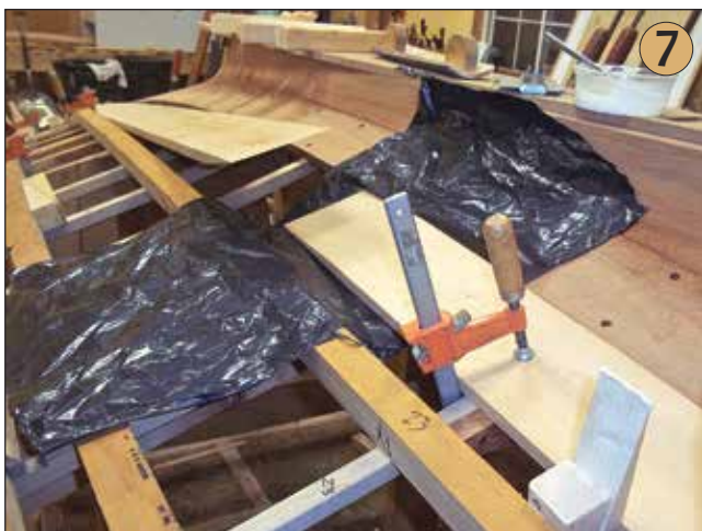
Photograph 7 —The broadstrake is made from two shorter planks scarfed together in place on the boat. Photograph 8 —The completed plank scarf. When faired, sanded, and painted, the joint will be invisible and secure.
