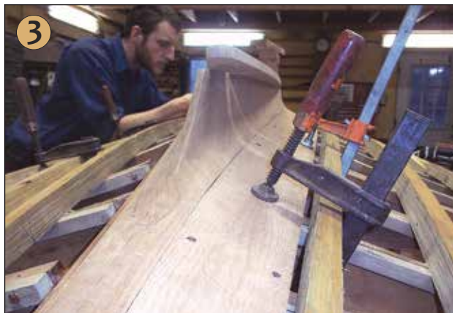
Photograph 1 —The setup: Each third frame is laminated to its precise shape, and permanent bulkheads are in place. Boatbuilders will note the absence of temporary molds. Photograph 2 —The rabbet has been cut in the laminated mahogany keel, and intermittent steam-bent frames are now in place. Photograph 3 —The garboard has been spiled and cut to shape, and glued and screwed into place.
