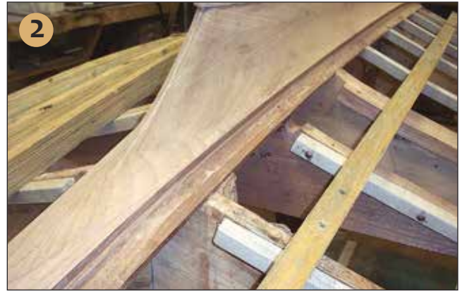
Photograph 1 —The setup: Each third frame is laminated to its precise shape, and permanent bulkheads are in place. Boatbuilders will note the absence of temporary molds. Photograph 2 —The rabbet has been cut in the laminated mahogany keel, and intermittent steam-bent frames are now in place. Photograph 3 —The garboard has been spiled and cut to shape, and glued and screwed into place.
