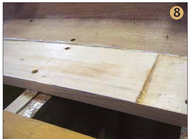
Photograph 7 —The broadstrake is made from two shorter planks scarfed together in place on the boat. Photograph 8 —The completed plank scarf. When faired, sanded, and painted, the joint will be invisible and secure.
