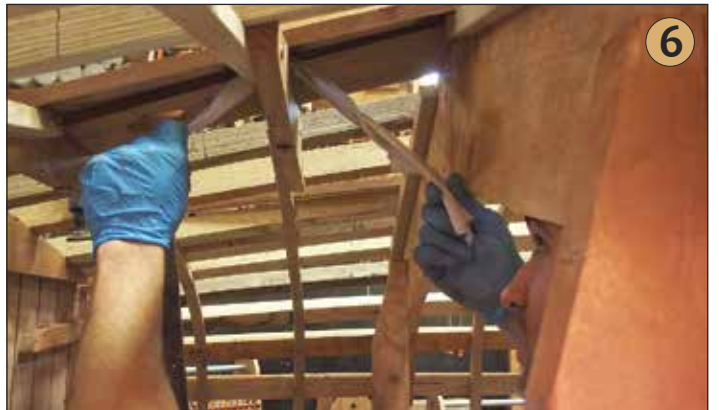
Photograph 4 —Wedges are driven between a hefty ribband and the glued-in-place garboard, driving the plank tight into the keel rabbet. Photograph 5 —The cedar broadstrake is glued and screwed in place. Photograph 6 —Excess glue is cleaned from the interior as well as from the limber holes in the floor timbers.
